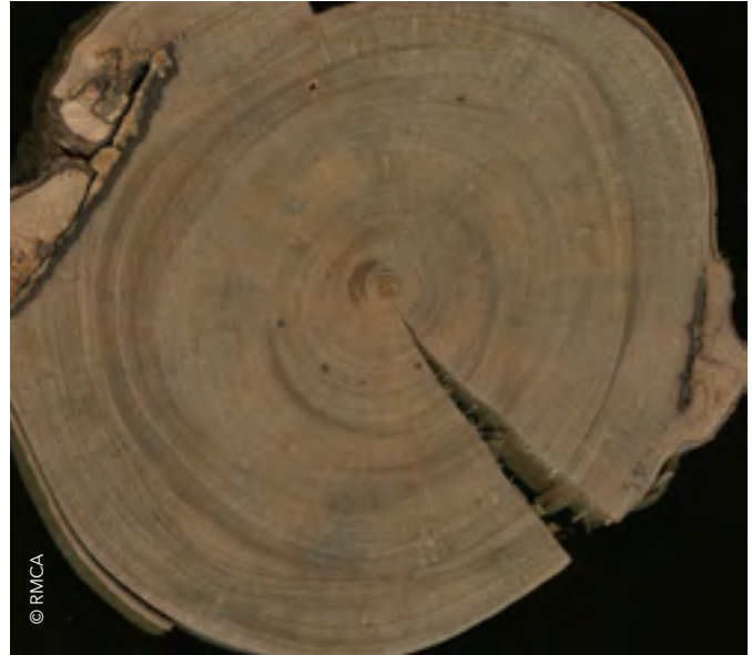
The 'SmartWoodID' project compiles an image database of Congolese wood species from the Tervuren xylarium. These images are used to identify wood based on macroscopic features with the help of artificial intelligence. Shown in photo: Prioria balsamifera (tola).
