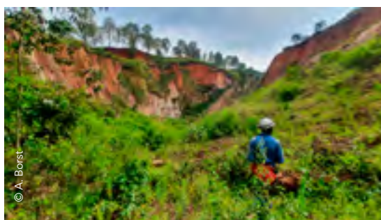
Abandoned open pit at Ntungwa, Rwanda, until recently mined for tin and tantalum from weathered pegmatites. Mining and exploration currently continues in underground tunnels.
