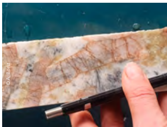
Drill core sample of a spodumene (lithium ore mineral)-rich pegmatite from Piran Rwanda Ltd operating in the Musha and Ntungwa area, Rwanda.
