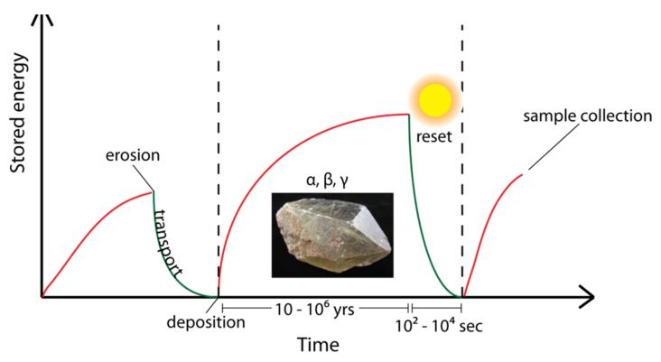
Fig. 1. Schematic view of the process of luminescence accumulation within sedimentary minerals.
