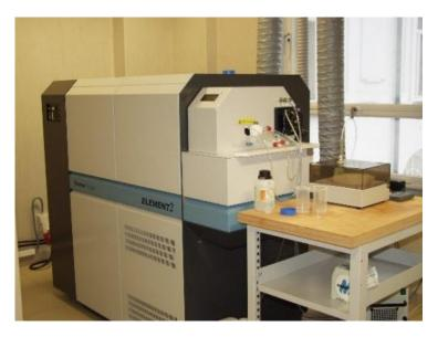
This instrument is a double focusing magnetic sector field ICP-MS with the main following characteristics:
